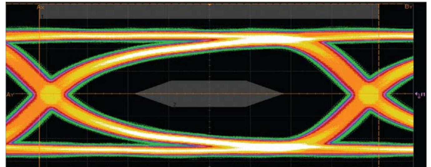
As clearly shown in this time domain eye diagram, NXP's robust PLL design provides significant design margin versus the JESD204A jitter mask specifications, helping to enable the extended rate and reach capabilities of the CGV implementation of this standard.
